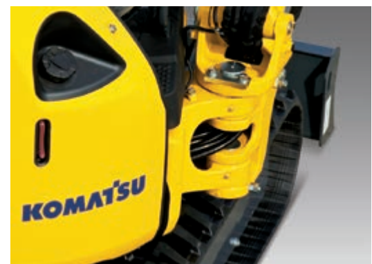
The swing cylinder has been relocated to the left hand side of the excavator to minimize protrusion so the operator doesn't have to worry about the cylinder when working near a wall.
